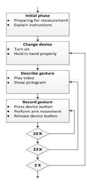
Fig. 3. Block diagram of the measurement. The described measurement consists of 10 repetitions of 23 gesture words by 2 mobile devices.
